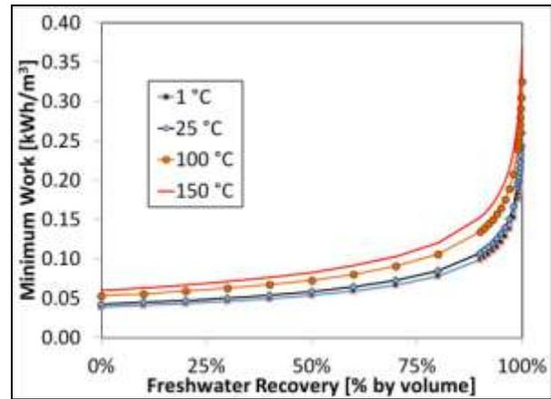
**Figure 2: Minimum reversible work required for isothermal desalination of 2‰ brackish water at common temperatures as a function of recovery.**
