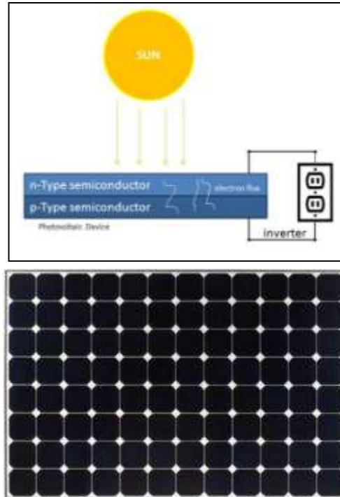
**Figure 7: (Top) Conceptual diagram of photovoltaic cell. (Bottom) SunPower WHT PV panel (source: SunPower).**
