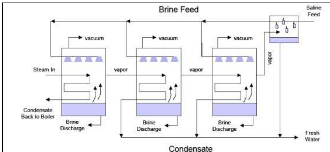
**Figure 4: Multi-effect distillation (MED) system diagram (source: PSA).**
