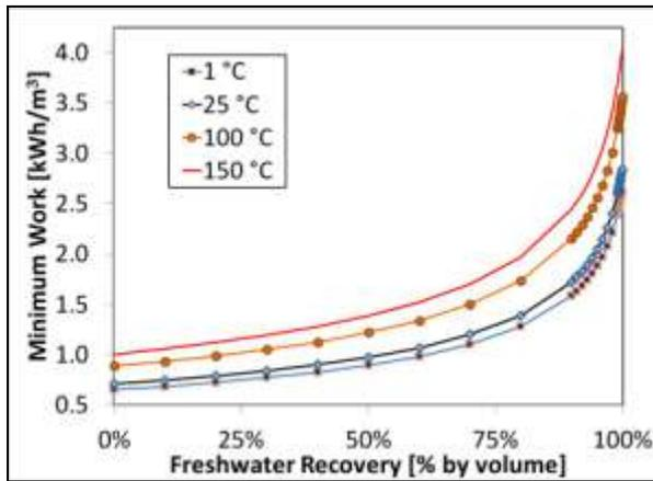
**Figure 1: Minimum reversible work required for isothermal desalination of 34.4‰ saltwater at common temperatures as a function of recovery. All liquid is removed at 100% recovery.**
