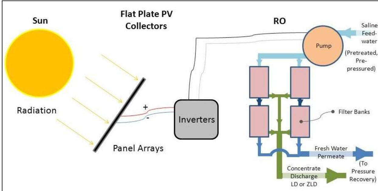
**Figure 9: Photovoltaic reverse osmosis (PV-RO) conceptual system diagram. Solar energy is collected by photovoltaic panels and converted to alternating current electricity. Saline feed-water is pumped through parallel filter banks, separating it into fresh water permeate and concentrate. Recovery devices transfer energy to the feed-water from both product streams. Concentrate is discharged or sent to a ZLD process. Permeate is treated and sent to consumers.**
