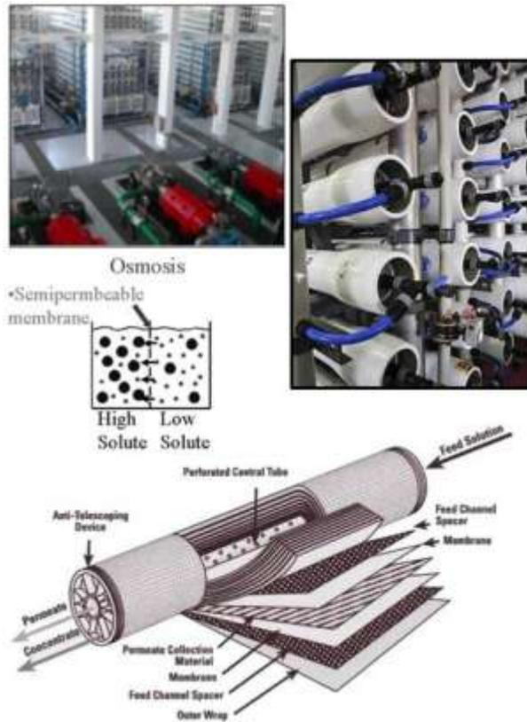
**Figure 3: (Top left) RO plant. (Top right) RO filter bank. (Middle Left) Osmotic flow with semipermeable membrane. (Bottom) Typical RO filter (source: DLR).**
