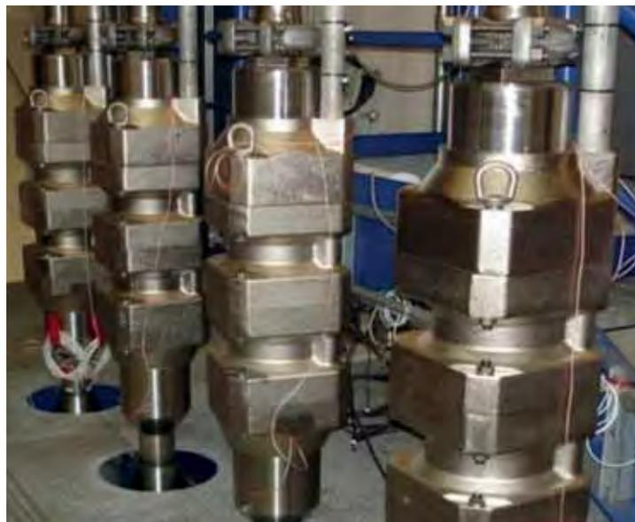
*Internal control rod drive mechanism testing.*
